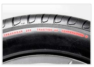
**TRACTION:** The traction grades, from highest to lowest, are AA, A, B, and C. These grades represent the tyre's ability to stop on wet roads as measured under controlled conditions on specified government test surfaces of asphalt and concrete. A tyre marked C may have poor traction performance. Caution: the traction grade assigned to the tyre is based on straight-ahead braking traction tests, and does not include acceleration, cornering, aquaplaning, or peak traction characteristics.
