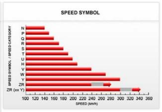
The Speed Symbol indicates the maximum speed at which the tyre can carry a load corresponding to its Load Index (except for loads at speed above 210km/h) under service conditions specified by the tyre manufacturer.
